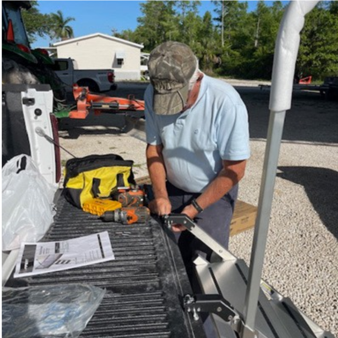
Getting the new truck ready for the next tour season – Charlie Egli and Tom Maish install a foldable ladder for safe access to the benches in the back of the truck. The newly installed foldable ladder will make the new benches in the back of the truck more easily accessible.
